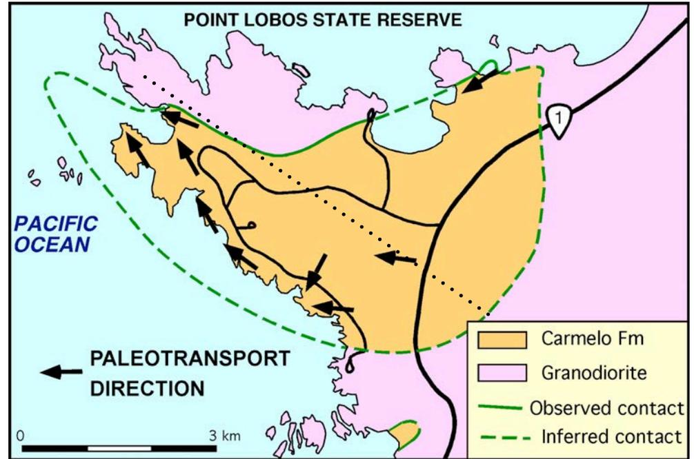
Figure 64. Distribution of the Carmelo Formation at Point Lobos and inferred direction of paleocurrents based on pebble imbrication and ripple marks and ripple lamination. Dotted line shows location of cross section shown in Figure 65.
