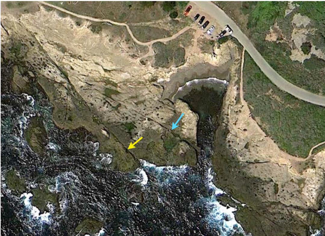
Figure 72. Prominent faults cutting across a rock platform on the South Shore between Weston Beach and The Slot. The eastern fault (blue arrow) displaces a couple of meters of strata: offset on the western fault (yellow arrow) is unknown, but may be in the range of 10 or more meters. Image from Google Earth.
