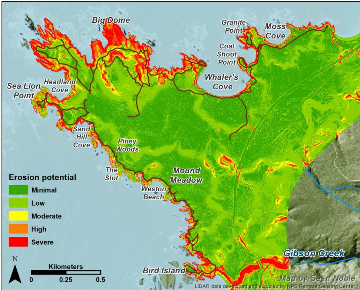
Figure 9: Erosion potential determined from topographic factors. This analysis does not account for variances in soil type or vegetation cover (Larger map available in Appendix B).
