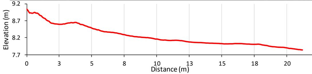
**Figure 29: Cross sections of the Slot 1 bluff from the photogrammetry survey. The areas that still have vegetation were approximated 0.1 – 0.2 m higher than the adjacent devegetated areas.**
