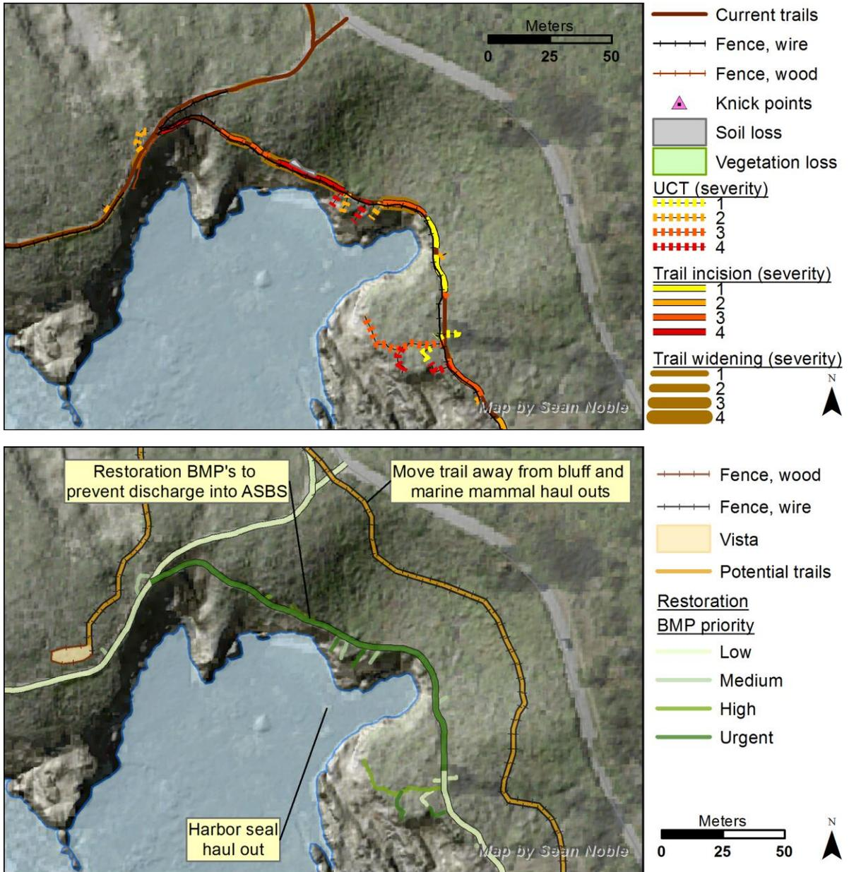
Figure 19: Suggested alternate trail paths around Sand Hill Cove. The vistas were chosen from the existing vista location and a point that has views of the Sand Hill Cove and the southern coast. The suggested trail does not account for orientation against slope and may be better positioned closer to the road.
