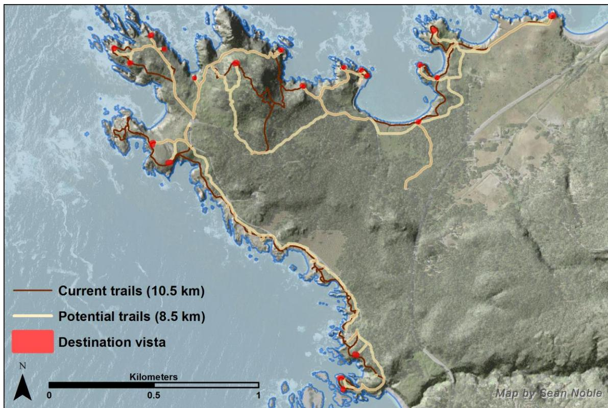
**Figure 17: Alternate trail paths as determined by a least cost analysis from the parking lots to selected vista points. The vista points were selected from existing vista location and areas that were the destinations of large numbers of UCT's. These trails do not take into account the orientation in respect of the hill slope.**
