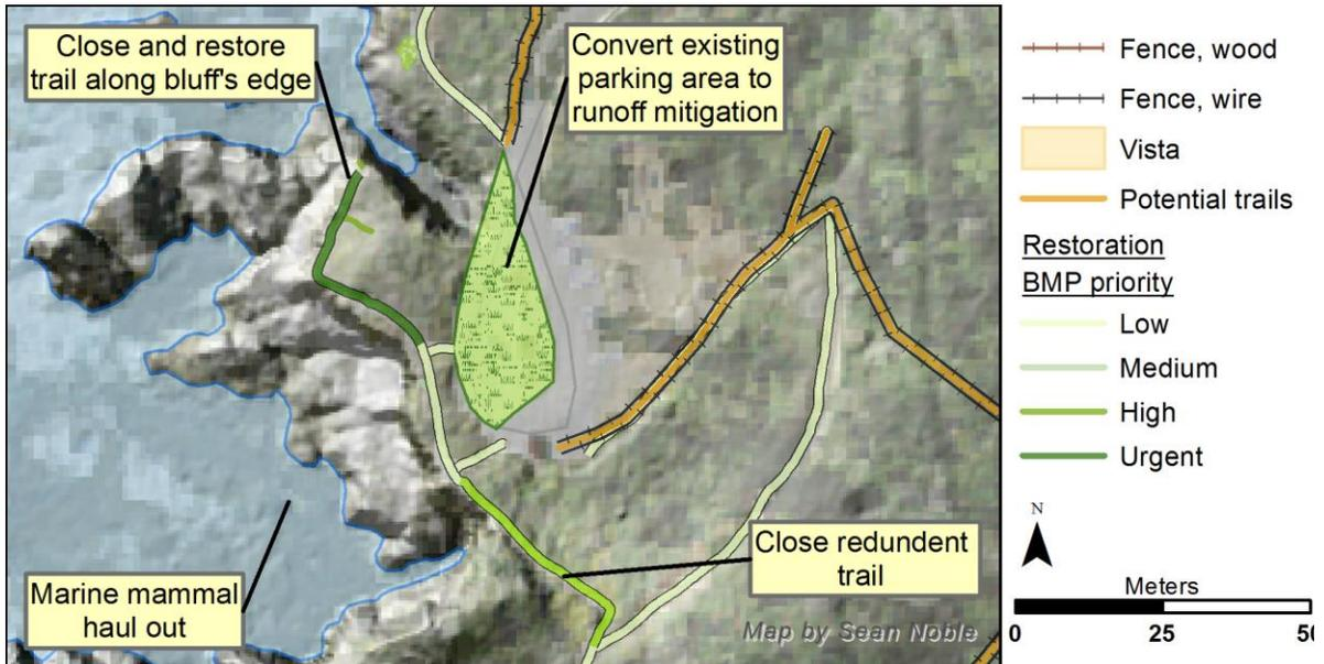
Figure 25: Suggested alternate design for the Bird Island parking area to avoid runoff into the ASBS. This would significantly reduce the amount of available parking in the area, but may be preferable to completely closing the parking lot. Significant research would have to be conducted to ensure that appropriate runoff mitigation could be implemented in the given space. Contrary to what the figure suggests using the existing ADA trail is preferable.
