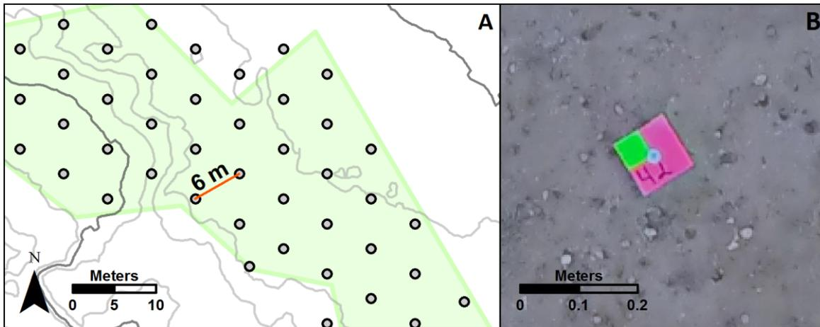
Figure 6: The planned distribution of GCP for structure through motion survey (A) and an example of one of the GCP's used (B). The spacing of the GCP's was determined through testing the viewing area from the GoPro camera from the height of the painter's pole. The multicolored pattern and numbering on the GCP's made photo identification in PhotoScan more efficient.
