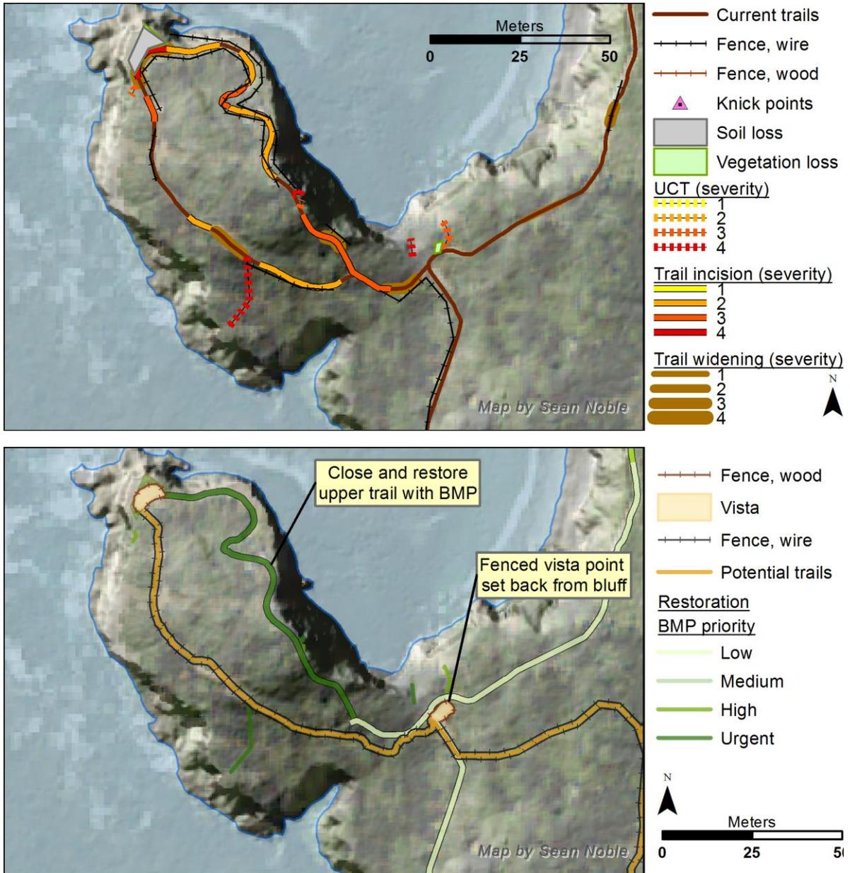
Figure 23: Suggested alternate trail paths on Coal Shoot Point. Closing the Northern section of trail would avoid most of the steeper section of the point. By fencing in a vista, a vegetated buffer can be implemented around the edge of the bluff.
