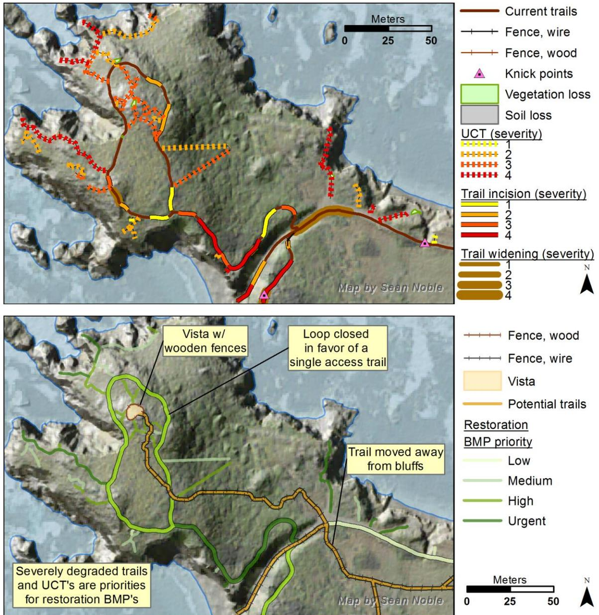
Figure 18: Suggested alternate trail paths around Granite Point. The vista point is location around a large rock at the peak on the point, which is the destination of most of the UCT's in the area.
