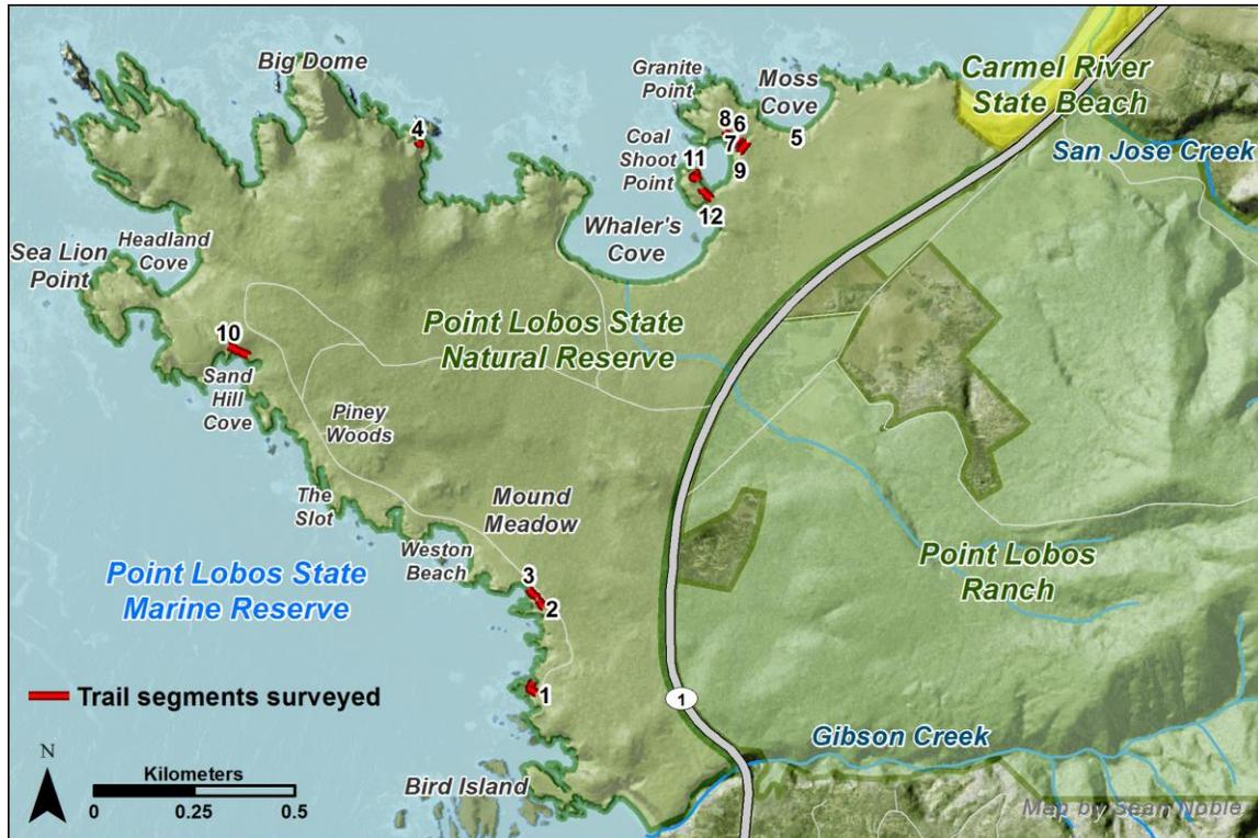
**Figure 4: Trail segments surveyed using cross-sectional area measurements. Numbering is based on the order in which the trails were surveyed, which was contingent on trail availability due to visitor usage. Some trails, like the one leading to Sea Lion Point, were selected in the GIS analysis, but were not surveyed due to the chance of disturbing marine mammals.**
