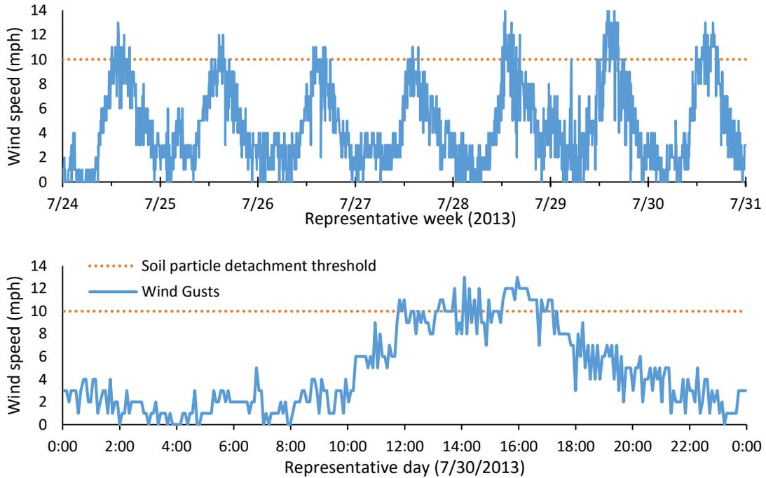
**Figure 8: Wind gust speed during a representative summer week and day of 2013. We compared the wind speed average and standard deviation to the yearly data to identify representative sections.**
