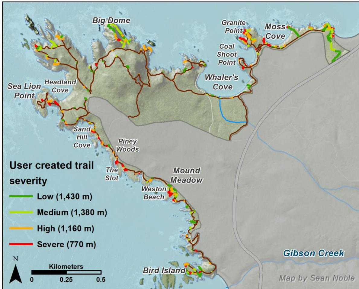
Figure 12: User created trails in the coastal region of PLSNR. Trail severity was based on level vegetation trampling, widening and incision (Larger map available in Appendix B).
